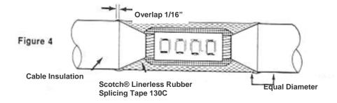
4.1 Smoothly fill in connector area with half-lapped, highly elongated Scotch® Tape130C; *BUILD UP TO DIAMETER OF CABLE INSULATION*, overlapping 1/16" (2 mm) beyond pencils. (Figure 4)
